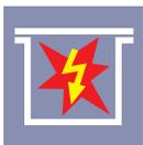
Although the North American term "explosionproof" and IEC term "flameproof" are SIMILAR concepts, the requirements in the product standards are different. Explosionproof is a Div. 1 technology which can be used in a NEC or CEC defined Zone 1 environment. Flameproof is a Zone 1 technology and can not be used in a Div. 1 environment.
